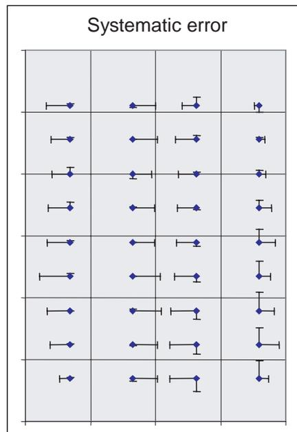
**Figure 3.** Systematic errors of images of a photogrammetric block with stripwise corrections for GPS observations (4 strips, 9 images/strip, 1 GCP in each corner and height control strips in 8 bases distances)
