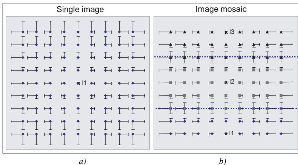
**Figure 2.** Geometric error of an orthophoto caused by 2 m height error. a) FLPIS orthophoto consisting of a single image; the maximum error is 1 m in both directions. b) FLPIS orthophoto mosaicked from 3 images (I1, I2, I3); dashed line shows the mosaic border; the maximum error is 1 m in X-direction and 0.6 m in Y-direction (flying direction).
