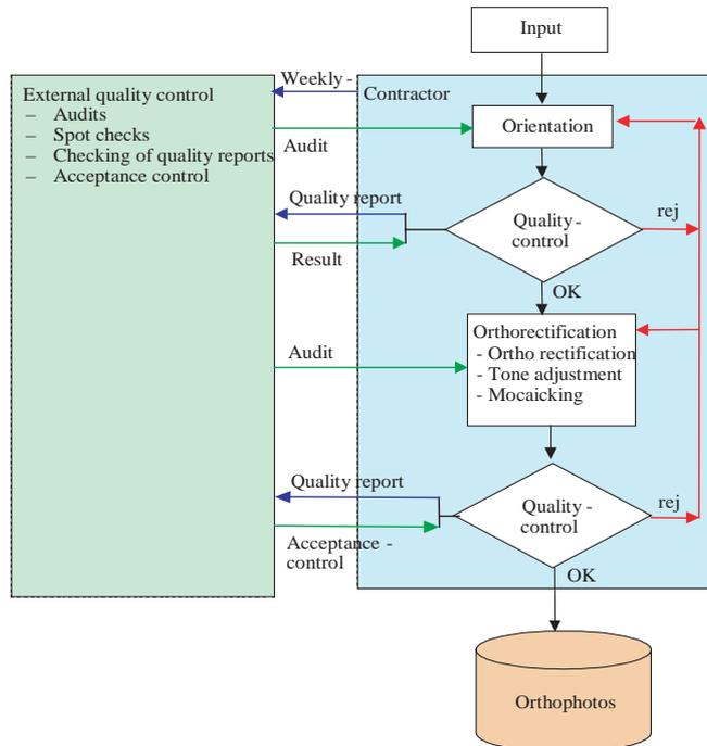
**Figure 1.** Digital image production, orthophoto production processes and QC
