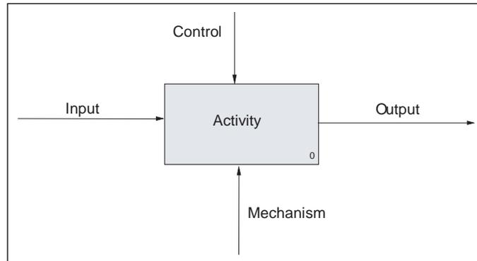
**Figure 1.** *The basic concepts of the IDEF0 syntax*
