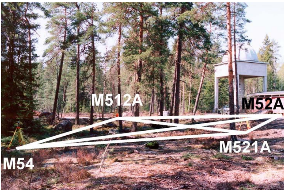
Figure 4. The four-points network for horizontal measurements in Metsähovi. (Photo Jorma Jokela).
