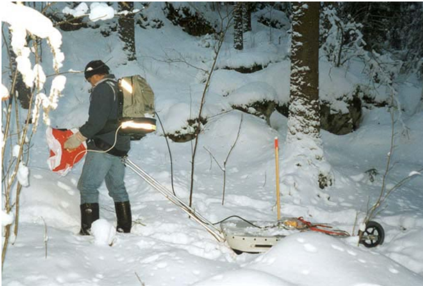
Figure 7. Ramac Ground Penetrating Radar in use.
