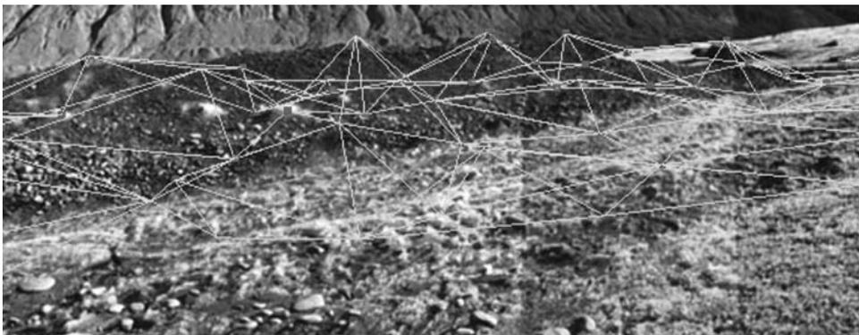
**Figure 5.** Triangulated laser scanner data projected onto one of the terrestrial panoramic images after IPP matching. Hintereisferner, September 2002.
