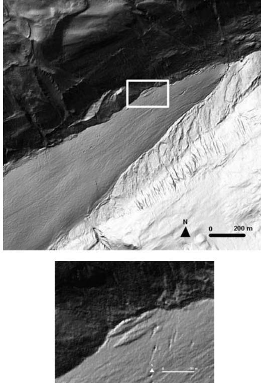
**Figure 2.** Hillshade of the DEM (cell size 1 m) derived from laser scanner data showing the tongue of Hintereisferner (above). Below is an enlargement from the upper image with a white frame indicating the place of the TP DEMs used in this study.
