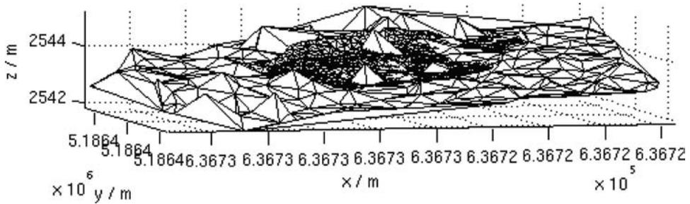
**Figure 4b.** Terrestrial photography DEM and triangulated laser scanner data after ICP matching. Hintereisferner, September 2002.
