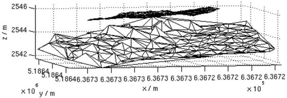
**Figure 4a.** Terrestrial photography DEM and triangulated laser scanner data according to the original georeferencing. Hintereisferner, September 2002.
