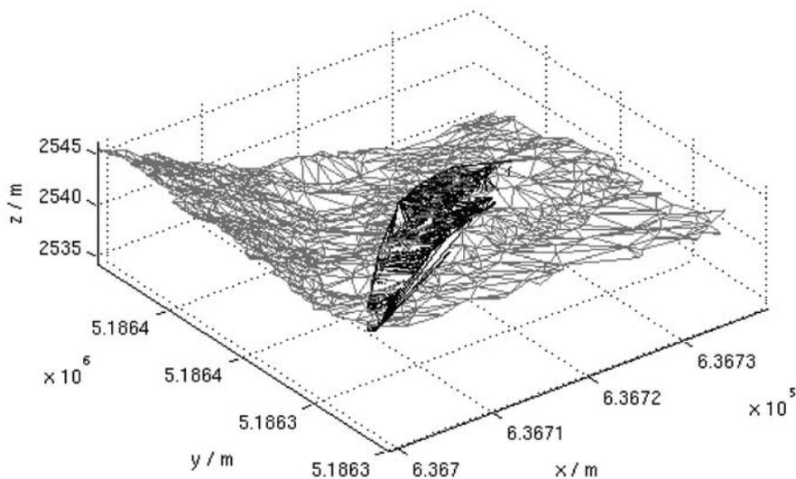
**Figure 6a.** Terrestrial photography DEM and triangulated laser scanner data after IPP matching. Hintereisferner, August 2003.
