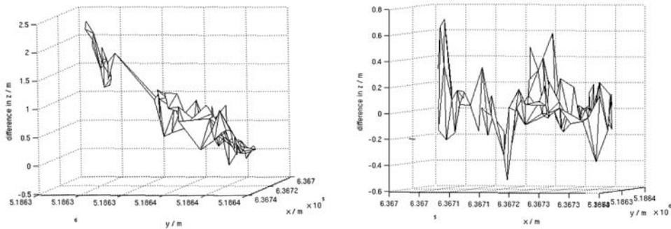
**Figure 7.** Elevations of the terrestrial photography DEM minus elevations of the triangulated laser scanner data a) according to the original georeferencing and b) after IPP matching. Hintereisferner, August 2003.
